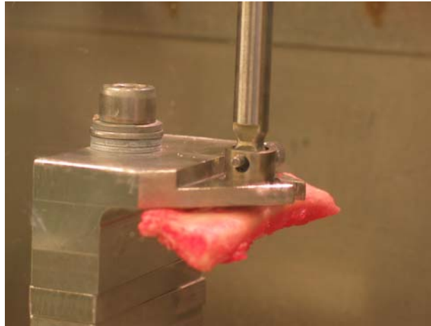
Figure 2. Pull-out test on Inion OTPS™ 2.5mm screws
