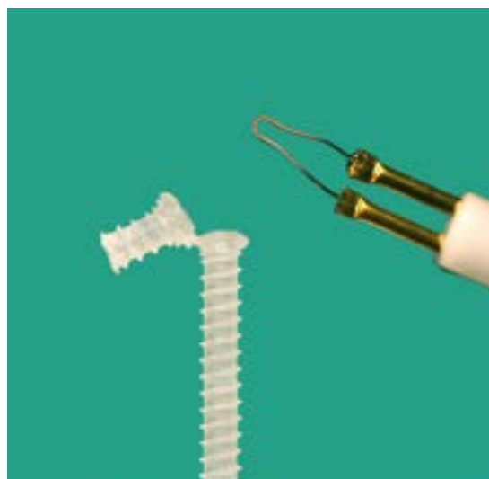
Memory Effect – ability to create new screw heads along the shaft by a low temperature hot loop
